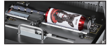
ROTARY UNIT Enables printing on cylindrical objects.
