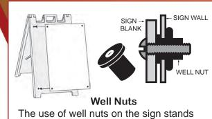
The use of well nuts on the sign stands makes changing signs easier by providing permanent mounting holes
