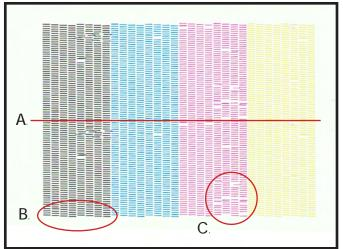
**Note:** If the pattern is missing just one or two nozzles this will not likely be noticeable in the printed image. This is because the printer uses multiple passes to create each image and each space will be covered multiple times depending on what print mode you are using. Higher quality print modes have more passes making missing nozzles less noticeable.
