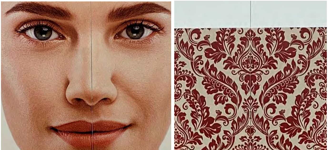
High resolution images showing dimensional and color consistency of wallpaper panels from beginning of the roll – panel 1 (left side) to end of roll – panel 13 (right)
