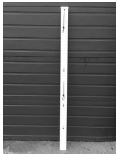
Photo 9: Shows post with top and bottom bungees interlocked in keyhole slots
