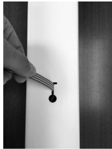
6: Pull bungee to top of keyhole slot and twist
