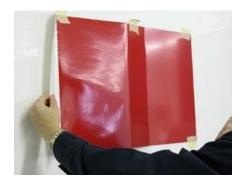
d) Re-squeegee the entire graphic using very firm squeegee pressure, including all edges. Puncture any air bubbles with a straight pin and re-squeegee from the edge of the bubble towards the puncture.
