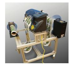
**The Gerber enVision Material Management System** maintains slack and rolls up the material after it is cut with the Gerber enVision 375. This system is designed to accommodate repeat cuts using sequence plot. The maximum single shape should not exceed 48" long when using both re-winders and sequence plot.
