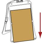
2. Slide through, pulling sign in front of bottom slot until sign hits the ground
