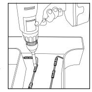
5. **Fasteners:** Use fasteners or silicone as necessary to fix modules in place. Refer to components list above for acceptable fasteners.
