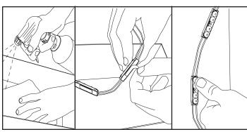
4. **Peel and stick:** Clean inside sign with rubbing alcohol and allow to dry. Using predetermined layout and LED placement from Step 3, remove tape backing and stick modules into place. Ensure modules are firmly attached. Other means of securing strip (sealant, vinyl, etc.) are also acceptable.
