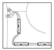
7. Cap all unused wires: Using appropriate UL Listed wire connectors (refer to components list on page 1), cap all used wires. Strand of modules should not be looped to create a close circuit.
