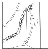
8. Connect power supply to first module on string: See power supply install guide for more information regarding power supply installation.
