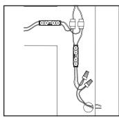
6. Connections: Modules may be connected in series\* or parallel.
