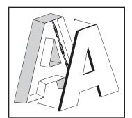
9. Replace sign face: Clean any debris from inside of sign and replace the sign face.
