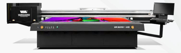
The VK3220T-HS redefines the meaning of productivity on a 3.2 x 2 meter (126" x 80") UV-LED flatbed. With up to three rows of printheads, print speeds can reach over 3,800 square feet per hour. Utilizing 4 picoliter drop size Kyocera heads and a high-speed magnetic drive, there's no compromise on speed to achieve remarkable quality. With the ability to print up to 10cm thick, the only limitation is your imagination.
