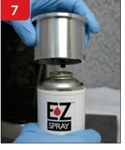
Insert metal cylinder cup on can's filling head; Insert plastic filling cup inside metal cylinder cup.
