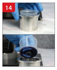
On flat non-skid surface, firmly press metal cup downward. This will pop plastic filling cup loose from metal cup.
