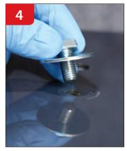
Secure the base plate to the machine with the provided short bolt (not long bolt) and washer through the center holes.
