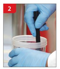
Prior to filling, thoroughly mix, shake and/or stir the paint.
