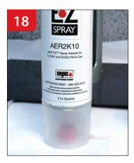
Place cap with red plunger on bottom of aerosol can.
