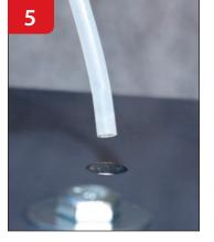
Thread air line for the machine through the bottom of the offset holes and up through the inside of the machine.
