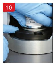
Rotate machine's turntable counter-clockwise until aerosol can is seated securely.
